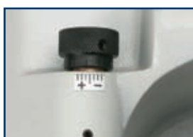
2 Tracer point with micrometric adjustment.
